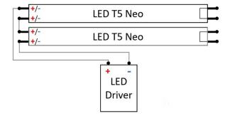
Due to the thermal conditions, only one of the two Neo lamps is connected to a thermocouple, as both lamps become equally warm during operation. When inserting the lamps, care must be taken not to tear off the thermocouples. A cable tie is sufficient for strain relief. Our driver is set to the highest current setting to measure the greatest possible heat generation. A functional test must then be carried out.
