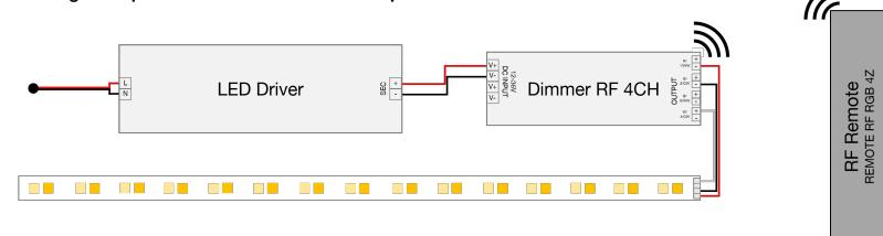
Wiring example for Tunable White LED Strips
