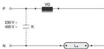
Standard circuit HID with internal ignitor
