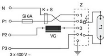
Circuit for 400V-HID-lamps suitable for hot restrike
