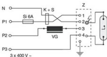
Circuit for 400V-HID-lamps suitable for hot restrike
