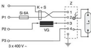
Circuit for 400V-HID-lamps suitable for hot restrike
