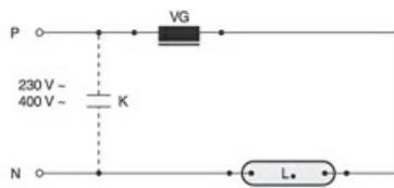
Standard circuit HID with internal ignitor
