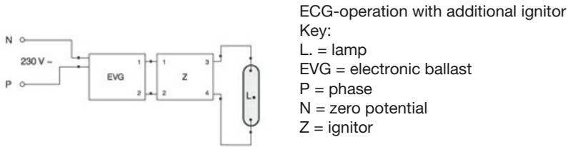
The required control gear (here ignitor and electronic ballast) for the lamps operation is usually mounted in the suitable luminaire in an appropriate electric circuit. Changes of any kind are to be conducted by qualified and specialised staff, only. Thus, this circuit example is to be understood merely as a technical background information for interested users.
