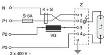
Circuit for 400V-HID-lamps suitable for hot restrike
