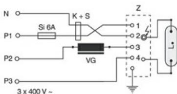
Circuit for 400V-HID-lamps suitable for hot restrike
