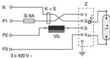
Circuit for 400V-HID-lamps suitable for hot restrike
