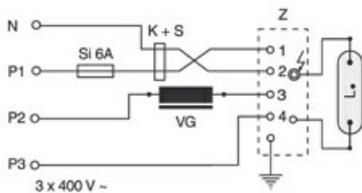
Circuit for 400V-HID-lamps suitable for hot restrike
