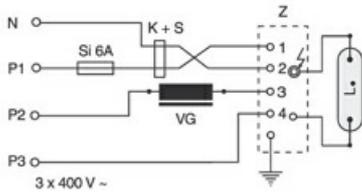
Circuit for 400V-HID-lamps suitable for hot restrike
