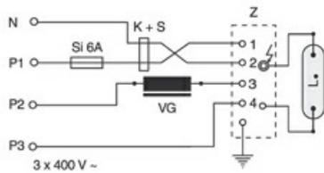
Circuit for 400V-HID-lamps suitable for hot restrike
