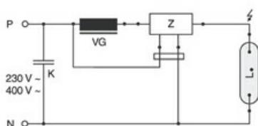
Circuit for 230V-HID-lamps suitable for hot restrike
