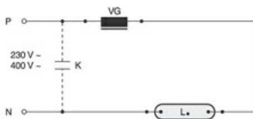
Standard circuit HID with internal ignitor
