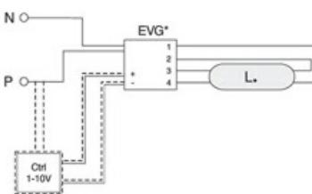
One-lampe circuit with electronic ballast
