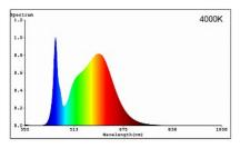
LED-NEO-Tubes 4000K, Replacements for fluorescent lamps
