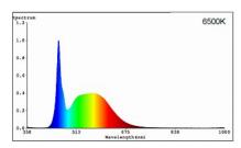
LED-NEO-Tubes 6500K, Replacements for fluorescent lamps
