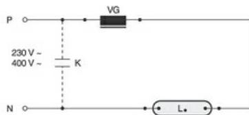
Standard circuit HID with internal ignitor
