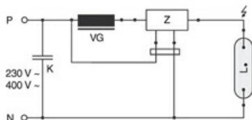
Circuit for 230V-HID-lamps suitable for hot restrike
