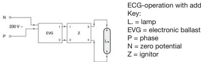
The required control gear (here ignitor and electronic ballast) for the lamps operation is usually mounted in the suitable luminaire in an appropriate electric circuit. Changes of any kind are to be conducted by qualified and specialised staff, only. Thus, this circuit example is to be understood merely as a technical background information for interested users.
