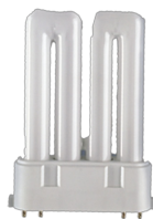
Lampe fluorescente compacte Ralux®Twin, RX-TW 24W/830/2G10
