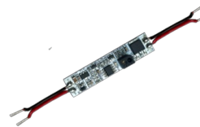
Build-in sensor for aluminium profiles, In-Profile WINK Sensor 96W/12-24V
